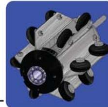
Guides for inspections to a minimum of ø400 mm
