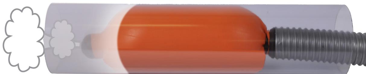
After connection the hose with the sealing bellows can be pushed into the pipe. Preferably provide for a smooth pipe wall to obtain optimal sealing. If the smoke generator is at operating temperature pressure can now be built up. The Easyseal will expand and fixate itself within the pipe, so that a complete sealing is obtained and further pressure build-up can take place.
